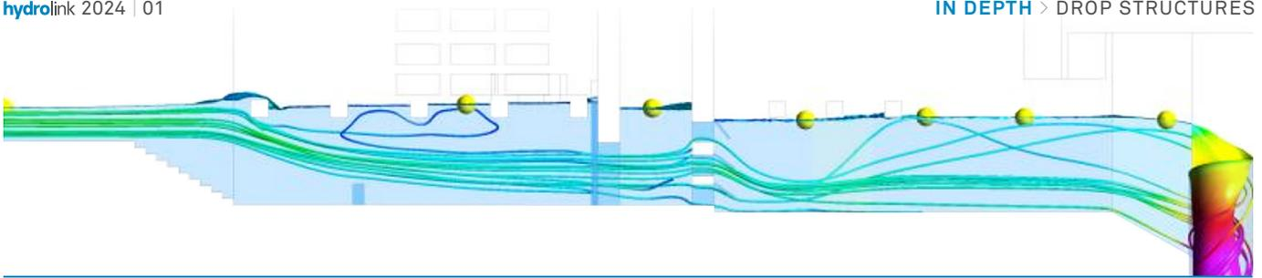
Figure 1 | Thames Tideway Tunnel CFD model used to develop initial designs.
