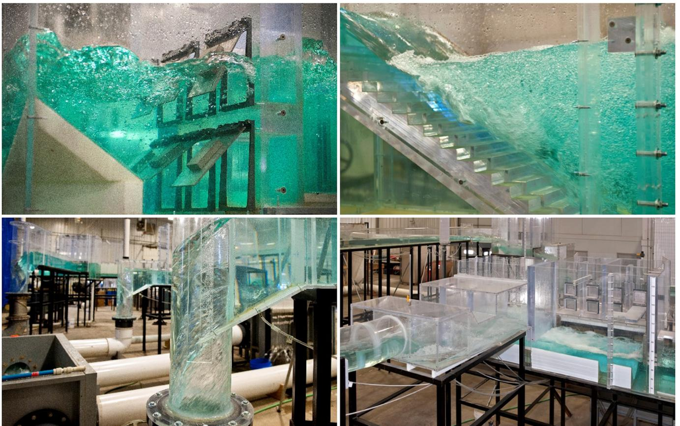
Figure 2 | Thames Tideway Tunnel 1:10 scale physical models used to improve and refine designs.
