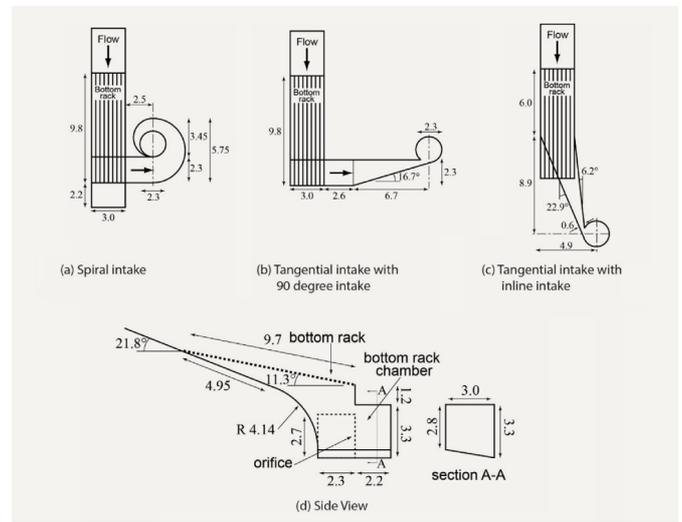
**Figure 3** | Integrated vortex intake designs for supercritical flow diversion (prototype dimensions shown in m).
