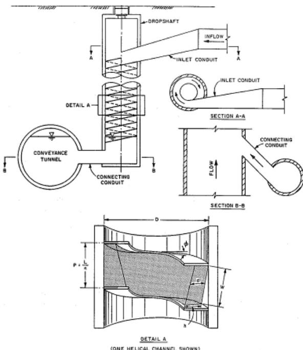
Figure 2 | Details of the helicoidal drop shafts in Kennedy *et al.* (1988).
