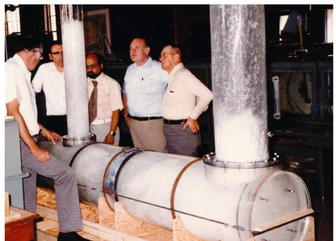
**Figure 1** | The large-scale, physical model of the tangential, vortex-flow intake and de-aeration tunnel. The model was used to aid the design of the Milwaukee drop shafts. The 1982 model included a tangential form of vortex-flow intake and a de-aeration outlet. (Image, courtesy of IIHR; Jain is in the middle of the group).
