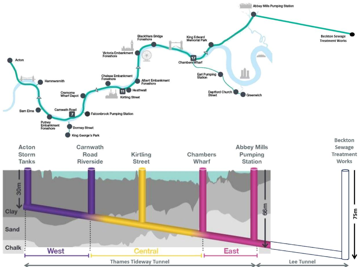
Figure 1 | London Tideway Tunnels route and sites with arrows indicating tunnel drive directions (top), main tunnel longitudinal schematic with drive/reception shafts and the prevailing geology (bottom).
