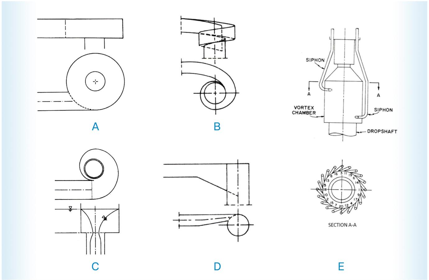
Figure 4 | Schematics of vortex-flow inlets for drop structures: (A) circular; (B) spiral; (C) scroll; (D) tangential; and (E) siphon<sup>8</sup>.
