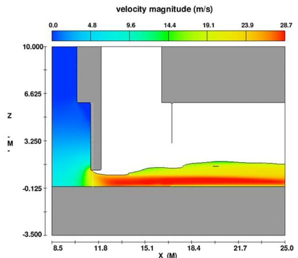
Figure 4 | Longitudinal profile of water level and velocities 4 minutes after start of gate opening.
