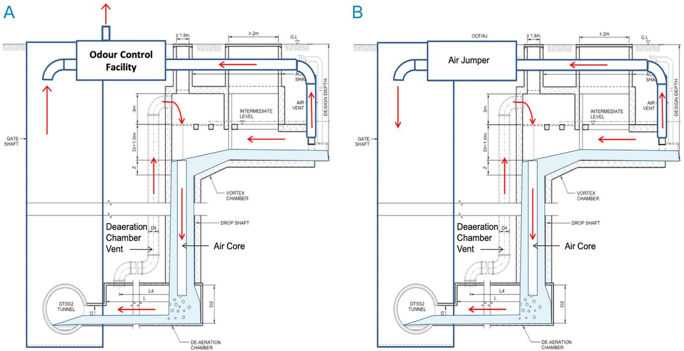
Figure 3 | (A) Odour Control Facility (OCF) and (B) Air Jumper (AJ) Schematics.
