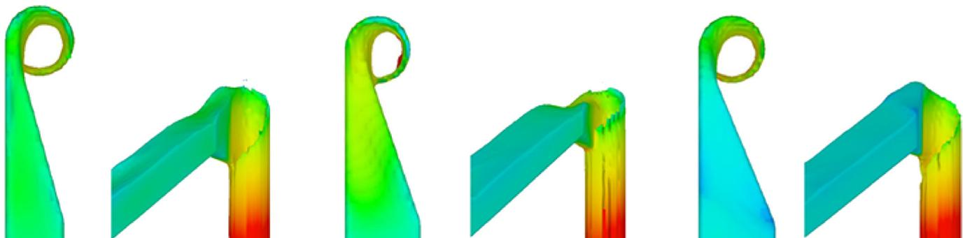
Figure 5 | Plan and elevation views from CFD modelling of several, approach-channel iterations (to tangential intake). (Image courtesy of AECOM).
