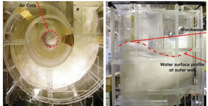
Figure 4 (B) | Spiral vortex intake with warp invert for supercritical flow diversion.
