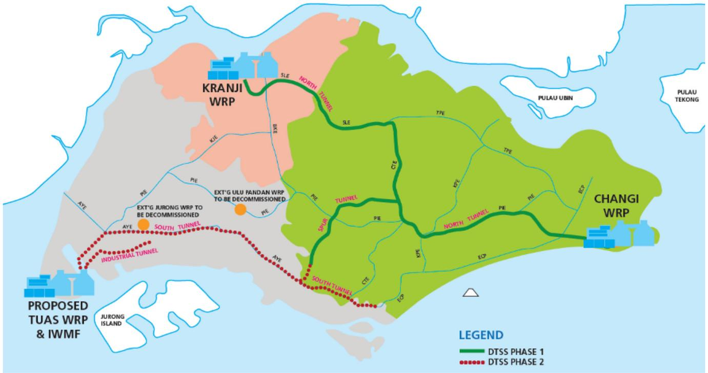
Figure 1 | DTSS Concept (WRP = Water Reclamation Plant, IWMF = Integrated Waste Management Facility).
