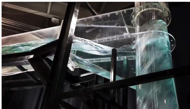
Figure 4 | The 1:16-scale hydraulic model of the tangential, vortex-flow intake used for the Forest Park Intake drop shaft. (Image courtesy of Jacqueline Stolze of IHR).
