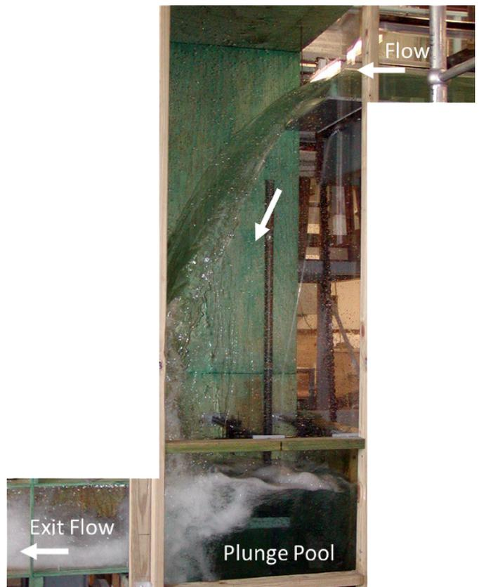
**Figure 2** | Laboratory testing of the hydraulic performance of a Roman, plunge-flow drop structure replicated at full scale (Chanson 2002).<sup>2</sup>
