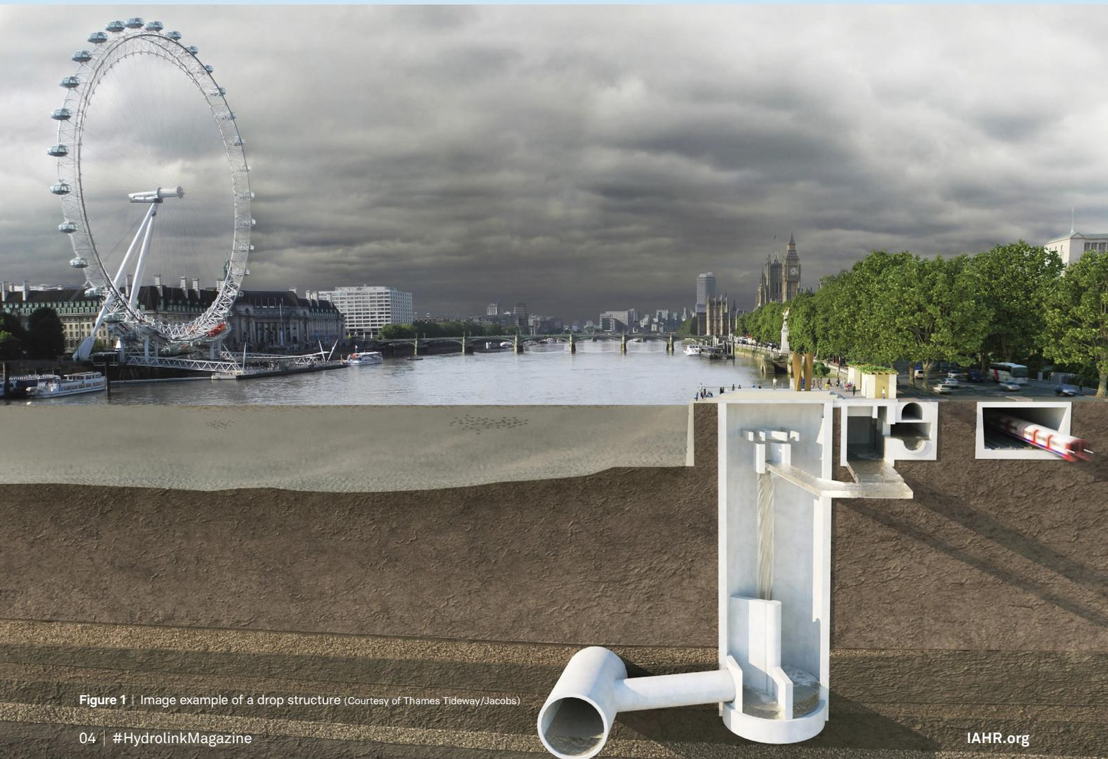
Figure 1 | Image example of a drop structure (Courtesy of Thames Tideway/Jacobs)
