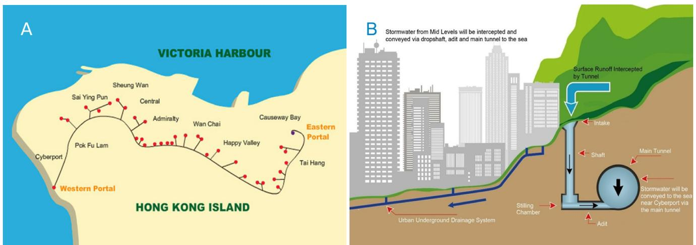
Figure 1 | Hong Kong West Drainage Tunnel System for urban flood management: (A) Layout of system of 34 supercritical vortex intakes; (B) upstream interception and diversion into tunnel.
