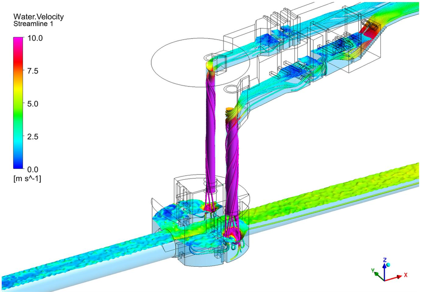
Figure 2 | CFD Model of TTT Dual Vortex Drop Interception Site (colour scale: water surface and streamlines coloured with water velocity [m/s]).
