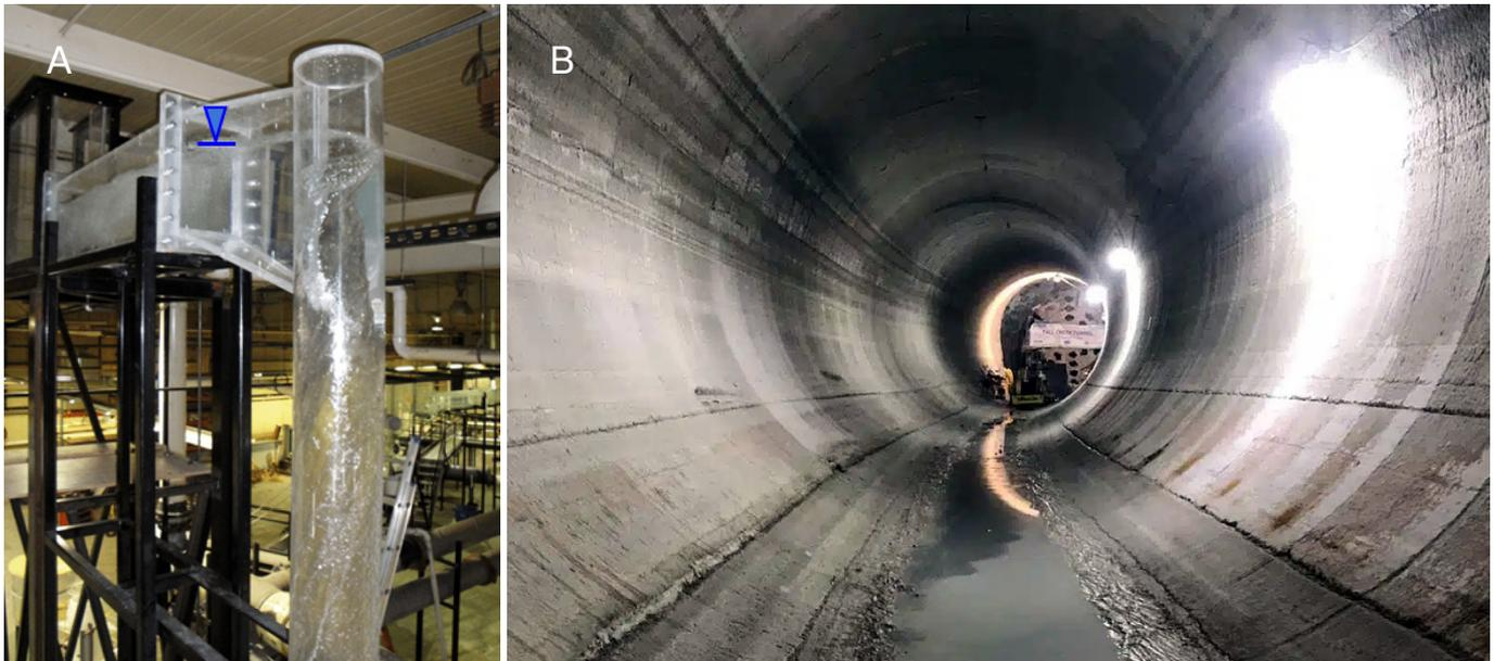
**Figure 6** | The 1:10 scale physical model of the tangential, vortex-flow intake, drop shaft, and tunnel for DigIndy Tunnel System: (A) operation of the drop shaft for a test run for the prototype flowrate of 15.8 m<sup>3</sup>/s (dropping 50.6 m in a 2.1 m diameter drop shaft); and (B) a view along one of the 5.5-meter diameter branch tunnels. (Photos courtesy of Troy Lyons of IIHR and AECOM).
