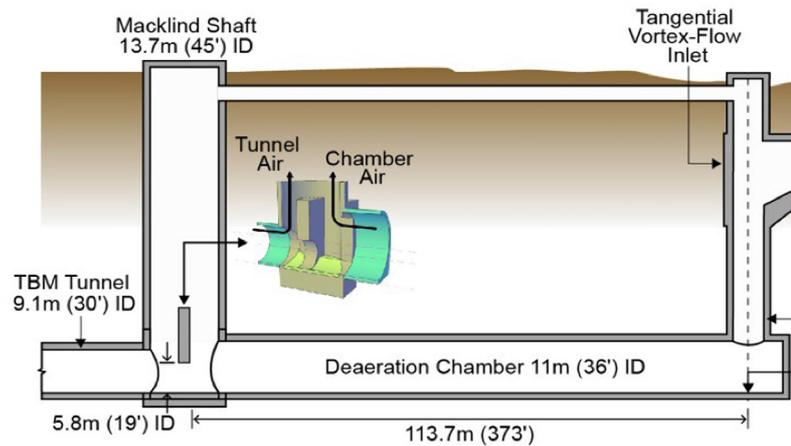
Figure 3 | Final layout configuration of the Forest Park Intake.
