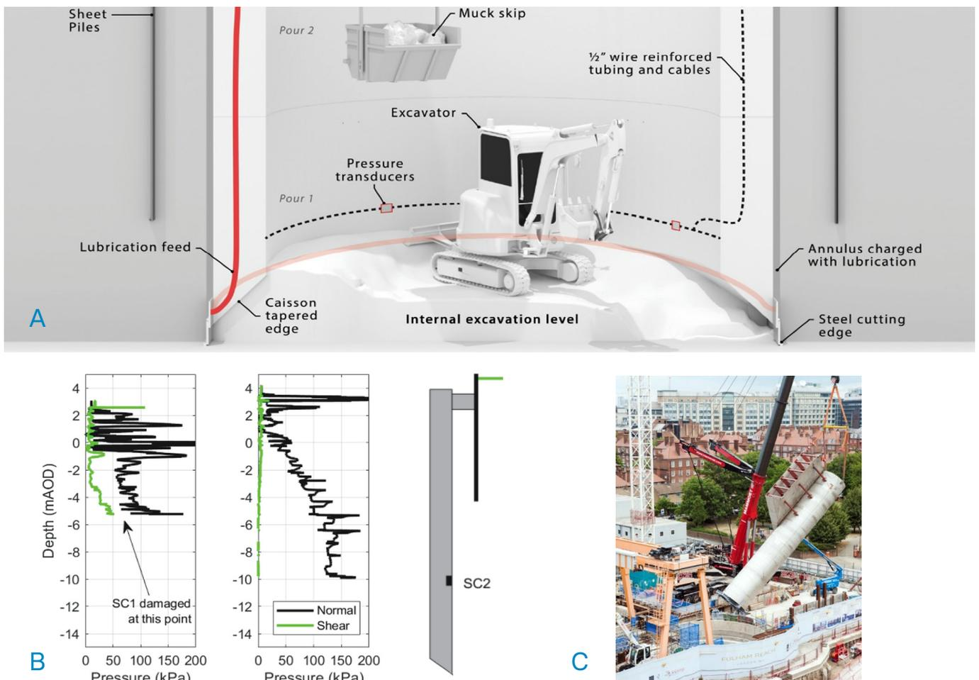
**Figure 5** | Examples of construction complexities: (A) and (B) Images from [www.wardandburke.com](http://www.wardandburke.com) on trenchless technology and shaft/caisson construction informed by pressure monitoring/machine learning (Courtesy of Ward and Burke); and (C) image of a stainless-steel tangential vortex generator and drop shaft liner being moved and lowered into position down the caisson shaft at Hammersmith, London. (Courtesy of Thames Tideway).
