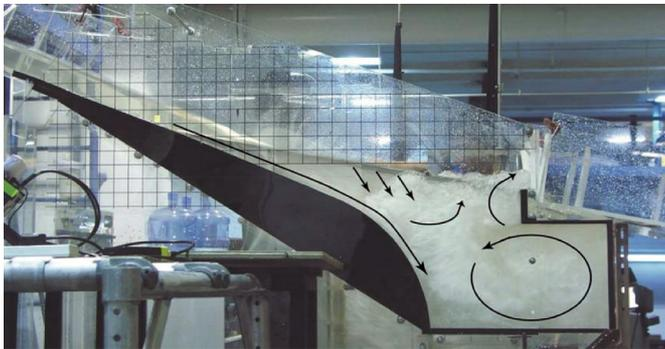
Figure 4 (A) | Bottom rack intake for supercritical flow diversion; observed flow at  $Q = 53.9$  l/s.
