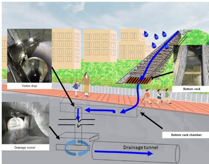
**Figure 2** | Design of integrated bottom rack-vortex intake system for stormwater interception (inset: constructed vortex drop and drainage tunnel).
