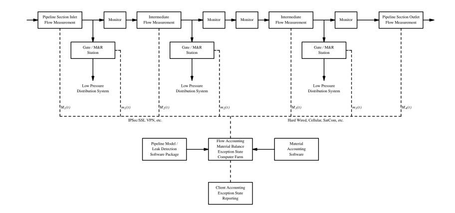
Upper case mass flows  $M_1(t)$ ,  $M_2(t)$ ,  $M_3(t)$ ,  $M_4(t)$  are high pressure Tranmission Pipeline Mass Flows. See Figure 1. Lower case mass flows  $m_1(t)$ ,  $m_2(t)$ ,  $m_3(t)$  are Outlet Mass Flows to low pressure Distribution System Pipelines. Transmission pipeline flow/state is monitored in same manner as in Figure 1.
