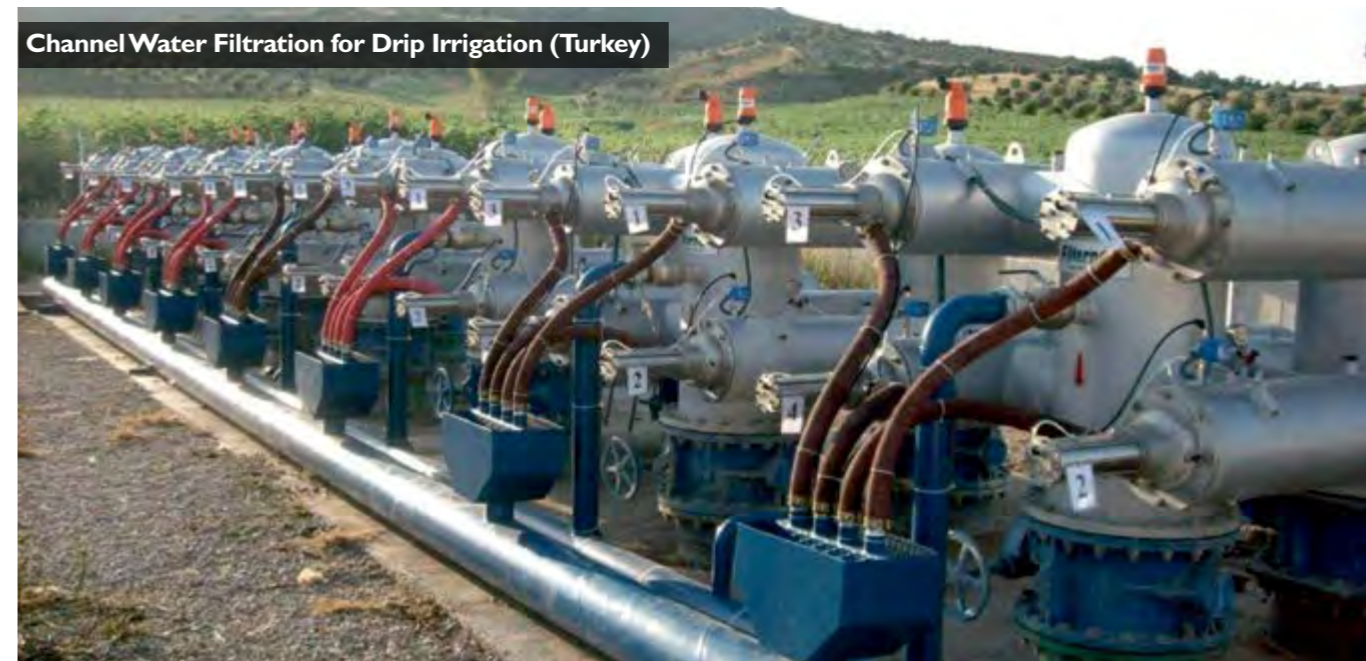
Well Water Filtration for Irrigation (Turkey)
