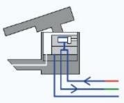
1 Push the lever down until it locks. The water is recycled to the inlet of the heater through a wide passage during a few seconds.
