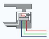
2 When the hot water reach the tap, a thermostatic element unlock the lever that will automatically return to neutral
