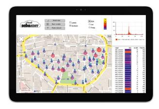
measurement data and track how the readings change over long periods. As well as this, you can save pipe network data, correlate measurement results and use network diagnostic functions.
