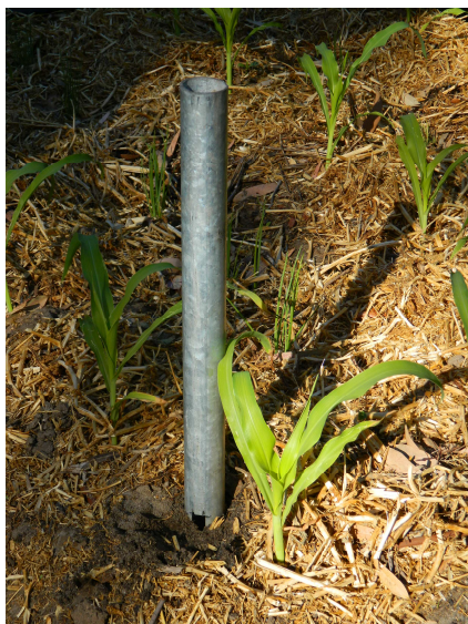
Early in the morning after irrigation the night before, push (or hammer) the steel pipe into the soil near a dripper.
