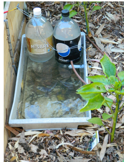
In this case 2 large drinking bottles have been used to adjust the surface area of evaporation.
