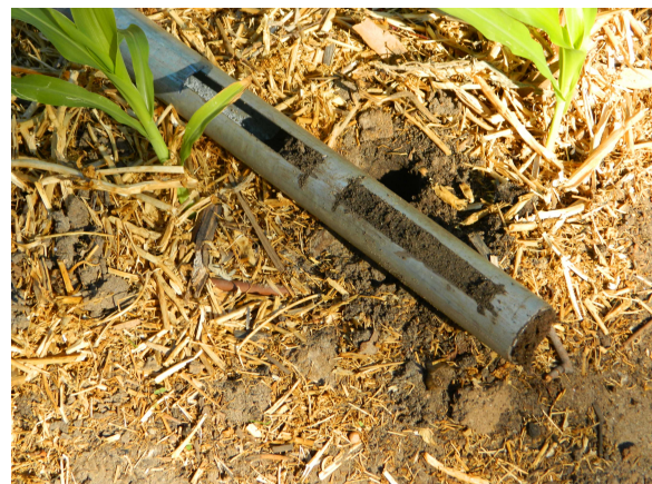
Remove the steel pipe from the soil and use the slots to inspect the moisture level in the soil and the position of the wetting front.
