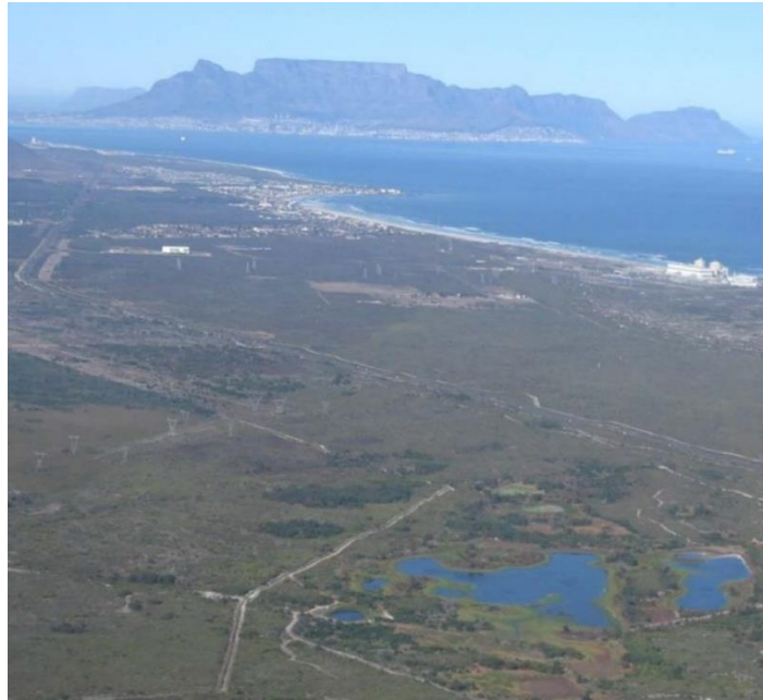
Figure 13 - Infiltration basins which form an integral part of the artificial recharge and recycling system in Atlantis. Cape Town's Table Mountain is in the background (DWAF, 2010).
