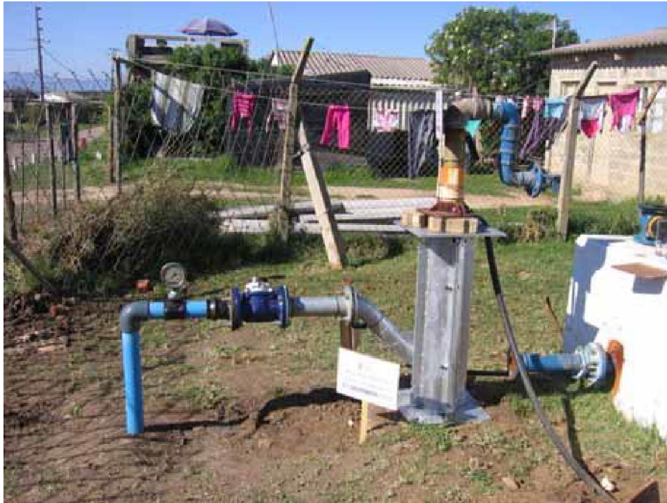
Figure 41 - Production borehole converted for conducting injection test (Murray and Ravenscroft, 2010).
