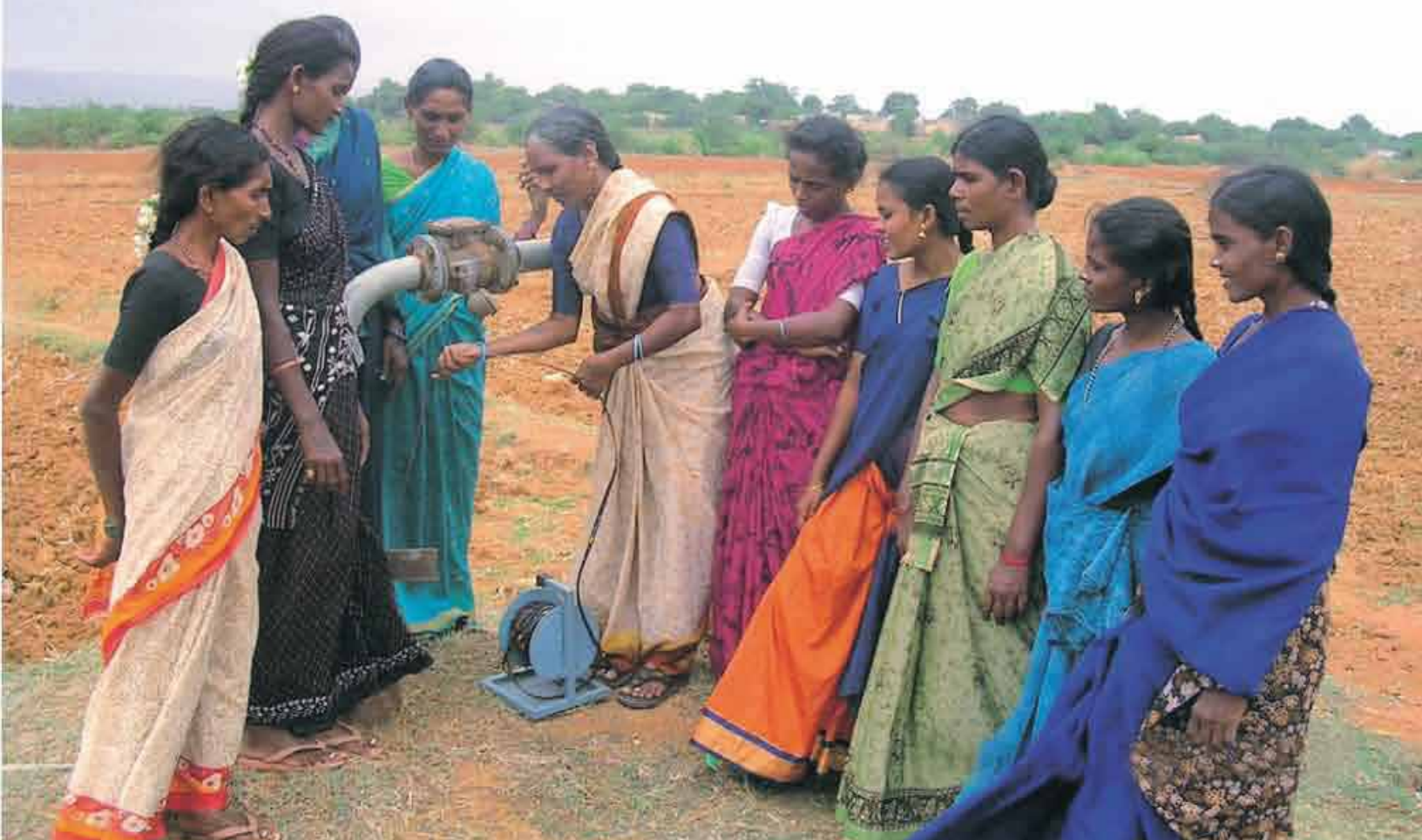
Sarojamma (center, holding the instrument) with other women farmers, using a water level indicator to measure groundwater level in an observation well. Sarojamma is data collection volunteer for Muthayalapadu village (Kurnool district, Andhra Pradesh)
