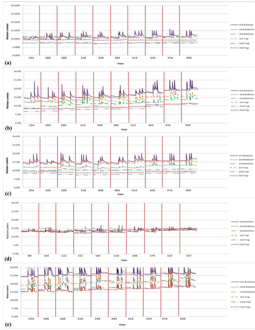
Figure 5. Moisture content of trench receiving (a) sanitary wastewater, (b) sanitary/kitchen wastewater, (c) sanitary/treated kitchen wastewater, (d) kitchen wastewater, and (e) treated kitchen wastewater – 10 min segments.
