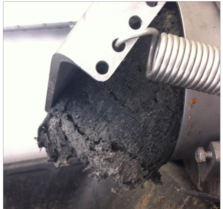
Compressed & dewatered tannery solids can be landfilled rather than discharged to biological processes or the sewer.
