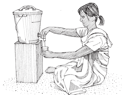
Figure 5.8. Tap fitted to a water bucket
