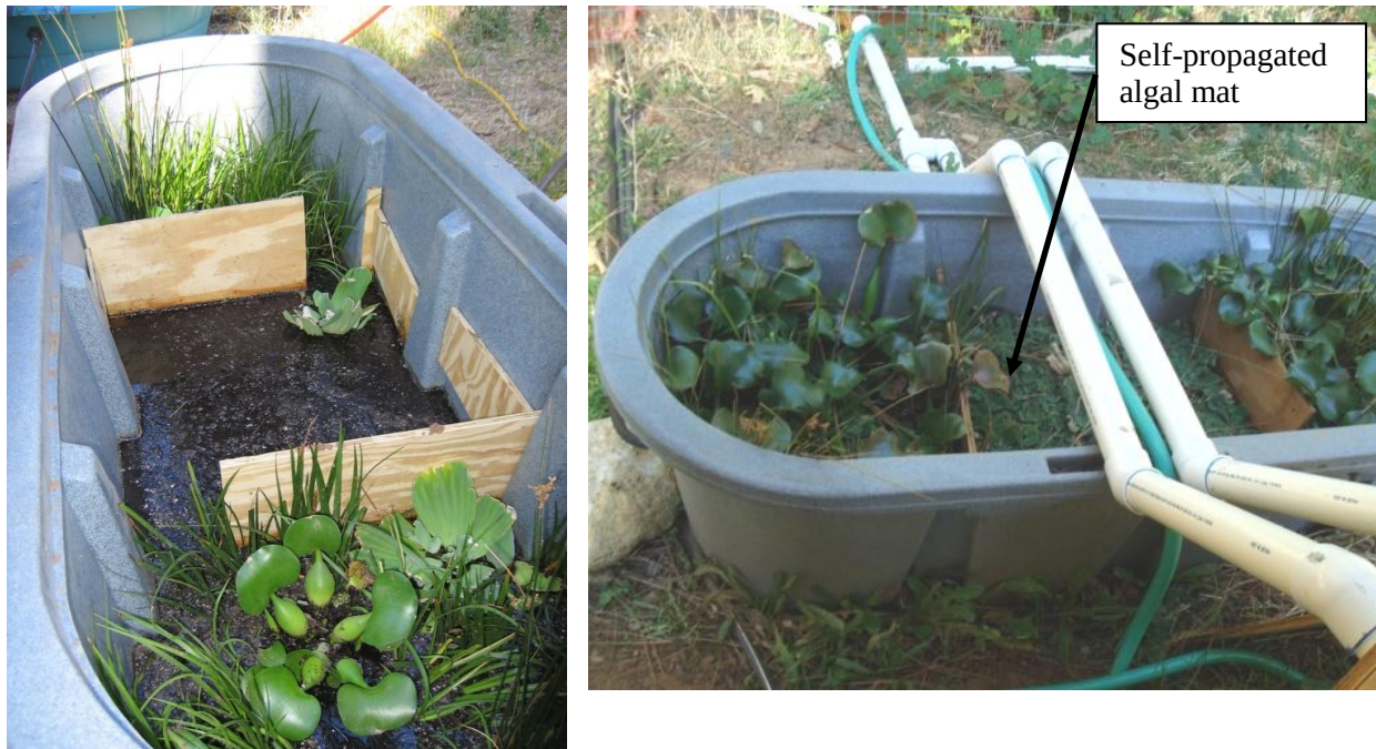
Figure 3. Initial (left) and 10-week-old (right) bench test wetland cells
