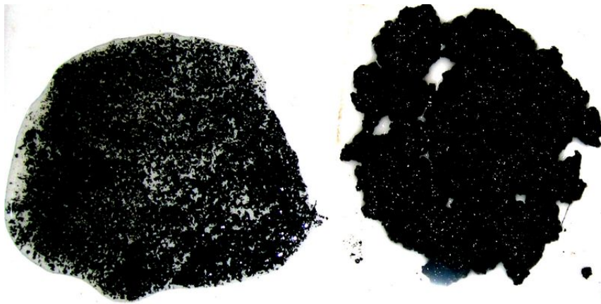
Waste Water before Separation (incl. Polymer): without with FloFormer
