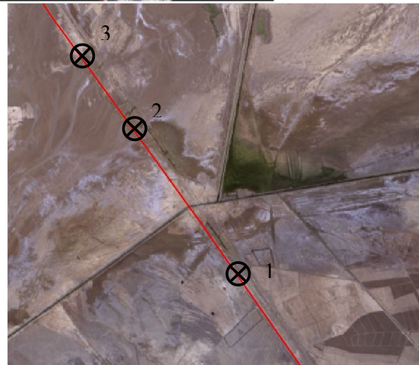
Fig. 2. (a) top: true-color Landsat 8 satellite image (Nov 06, 2014) over the Kosar water transmission pipeline, (b) left down: true-color image of leakage area (30-m pixel size) and (c) right down: pan sharpened image of leakage area (15-m pixel size).
