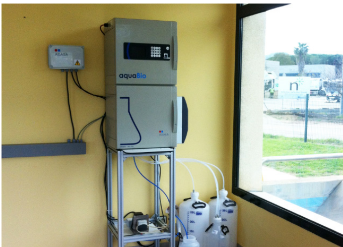
Figure 3. aquaBio, automatic E. coli analyser in water.
