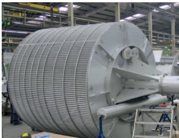
ROTAMAT® Perforated Plate Screen, 2600 mm diameter (6 units in total), 1 mm perforation
