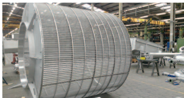
RPPS-Star screen basket, 2600 mm diameter, 1 mm perforation
