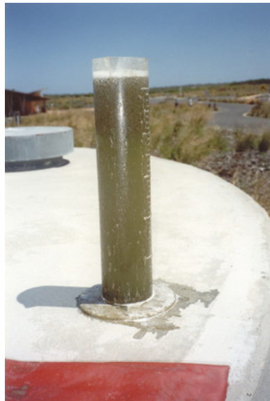
Cleaning liquor showing released sludge into the water column
