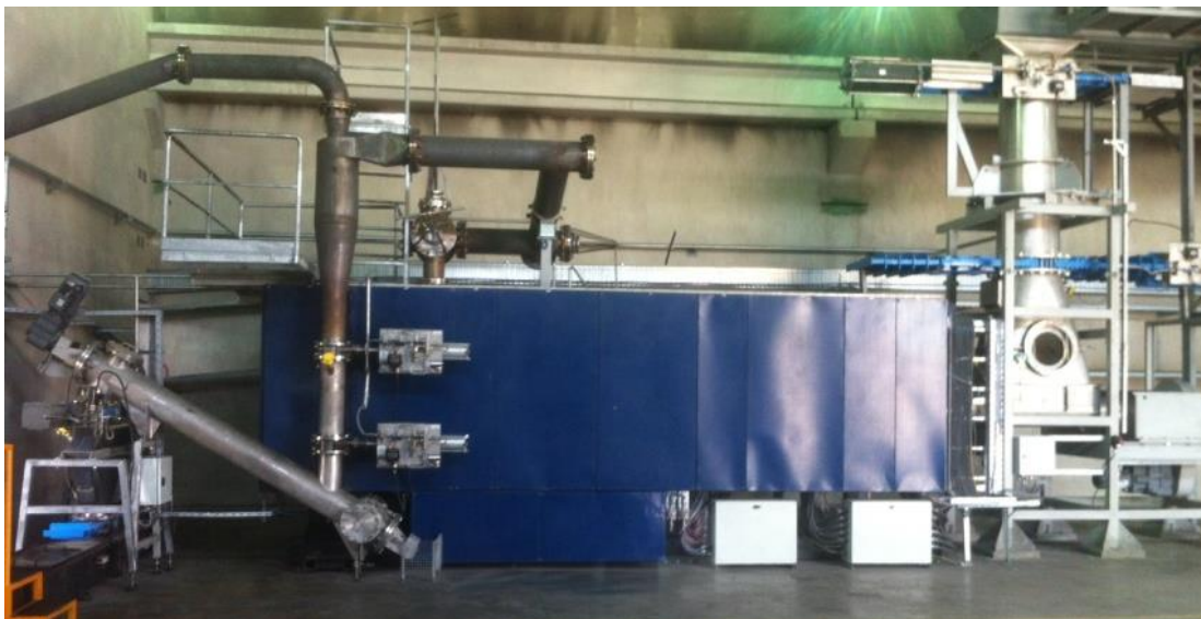
Figure 3 – A pyrolysis unit with a throughput of (15 Tonnes / day)
