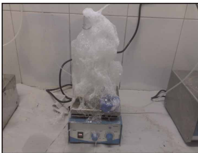
Figure 6 | Foaming during aeration optimization studies at 24 and 32 lpm/l aeration setups.
