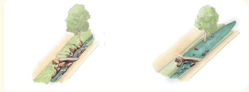
VEGETATIVE STONE SWALE - DRY AND WET
