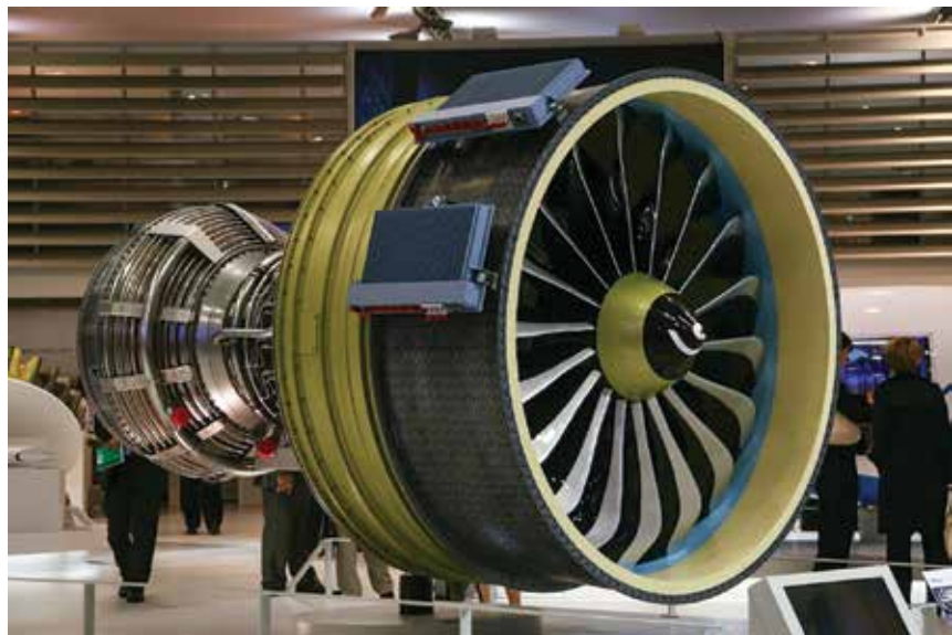
A full-size mockup of CFM LEAP-X. The LEAP aircraft engine is the first widely deployed CMC-containing jet turbine.
