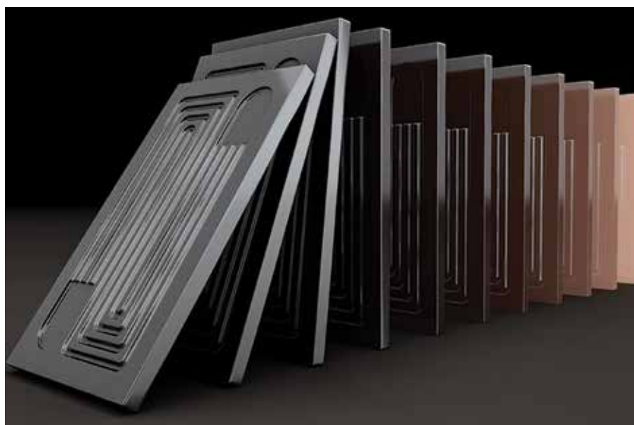
A team of researchers developed a ceramic-metal composite that would be cheaper to produce at scale than stainless steel or nickel alloy-based heat exchangers.
