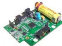
Fig 3. Acoustic Wireless Sensor
