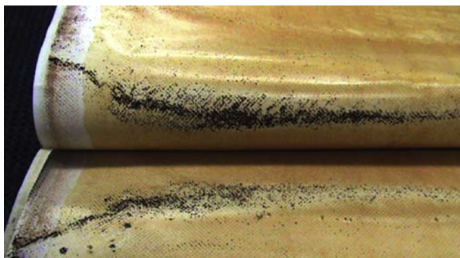
FIGURE 3.3 Accumulation of solids and organics on the membrane surface.
