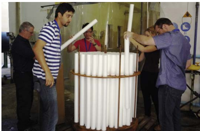
FIGURE 5.12 Cartridge filter loading.
