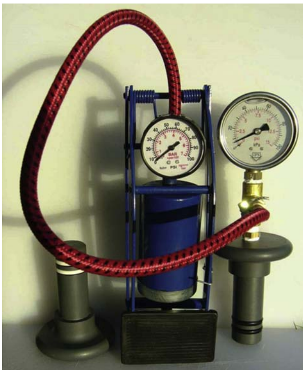
FIGURE 3.14 Bubble test equipment.
