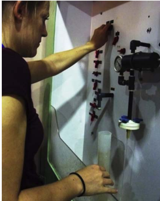
FIGURE 2.1 Typical SDI measurement device used in full-scale desalination plants.
