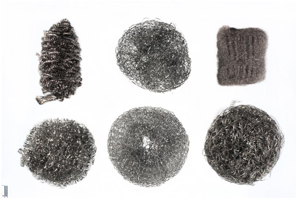
Figure 4: Photographs of six steel wool specimens found on the market in Douala/Cameroon (August 2015).
